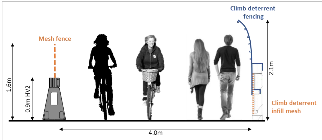
Figure 31 Proposed cross-section of Auckland Harbour Bridge Shared Path to address Waka Kotahi safety concerns (1.8m high people used for reference)
